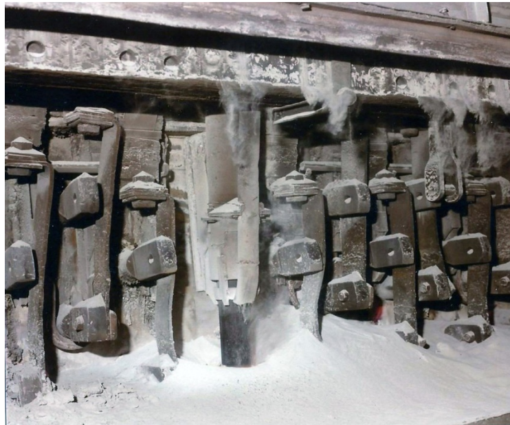
Fig. 9 Crust breaking and alumina feeding
