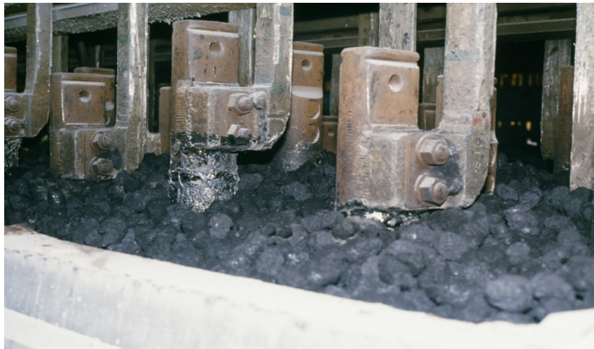
Fig.1 Dry anode mass on the anode top
