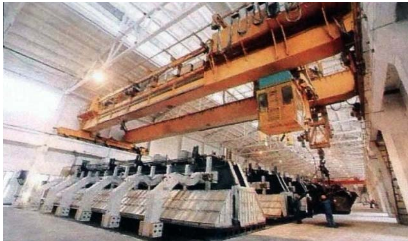
Fig. 10 Q-350 is the first Chinese-developed cell design with six risers
